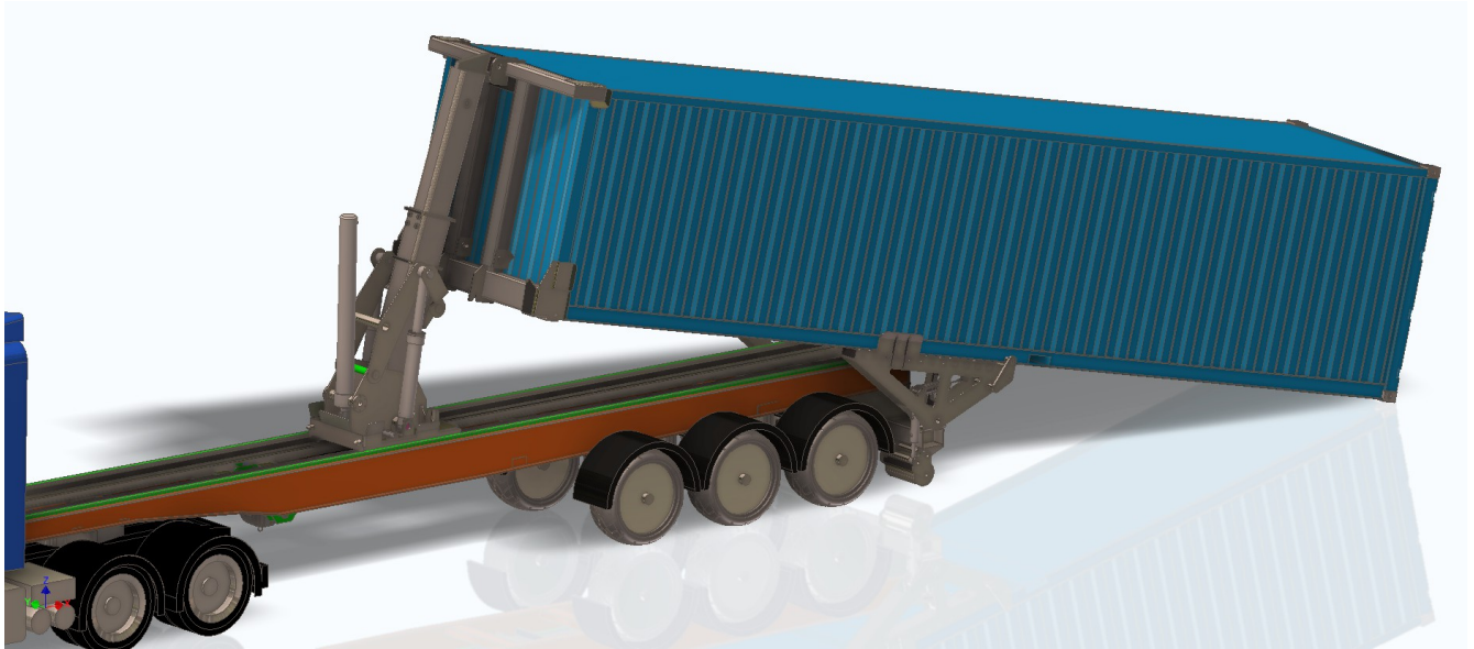
Pic. 3: 40' ISO Container Handling Unit ContiLift CHU-40 – Loading Mode
