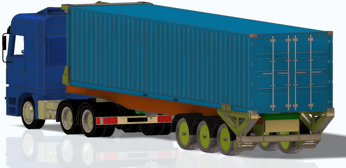
Pic. 1: 40' ISO Container Handling Unit ContiLift CHU-40 – Transport Mode
