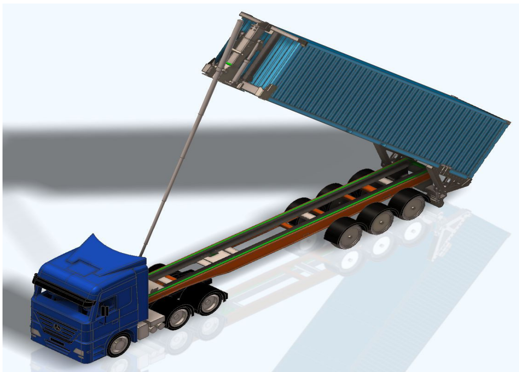
Pic. 2: 40' ISO Container Handling Unit ContiLift CHU-40 – Tilting Mode
