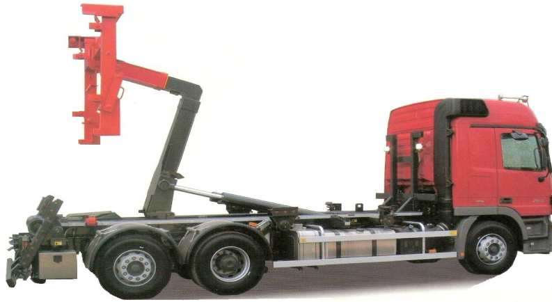
Pic. 1: EOS-ENVIRO Hook Lift SC 266 with Adapter Kit for 20' ISO Container
