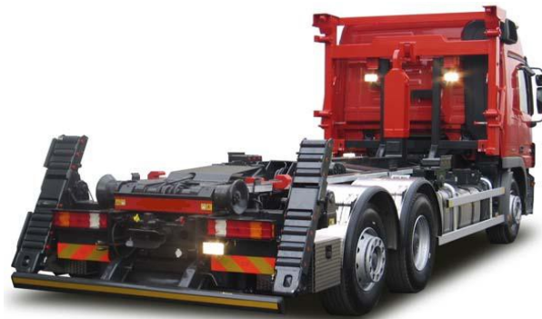
Pic. 5: EOS-ENVIRO Hook Lift SC 266 with Adapter Kit for 20' ISO Container
