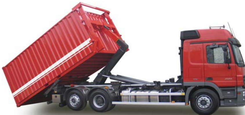
Pic. 2: EOS-ENVIRO Hook Lift SC 266 with Adapter Kit for 20' ISO Container
